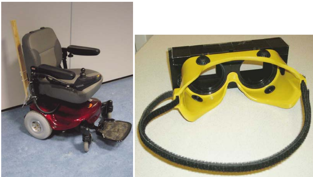
Figure 4: Left: the Electronic Wheelchair Used in the Control Conditions. The joystick is mounted at the end of the right armrest. Right: the tunnel vision goggles with the same rectangular fieldsize as the camera system in the remote control situation.
