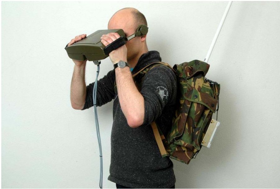
Figure 12: A Handheld Telepresence Interface that Allows the User to Steer the Remote Camera by a Device that Resembles a Pair of Binoculars.
