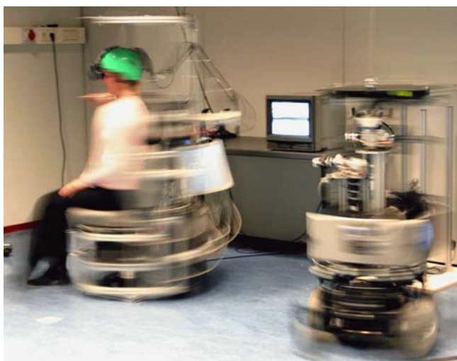
Figure 6: In the ROV Stepping around Control Condition, the Heading of the Remotely Operated Vehicle is Coupled to the Heading of the Operator's Chair. Stepping around thus controls vehicle heading.
